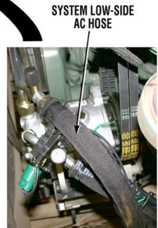
SYSTEM LOW-SIDE AC HOSE (AC EVAPORATOR CORE OUTPUT)
