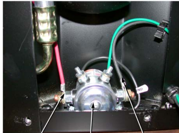
AC CONDENSER ASSEMBLY HARNESS BLACK WIRE
