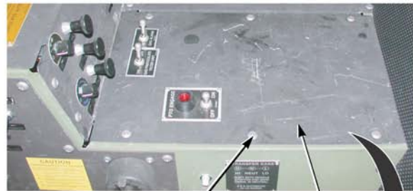
SCREWS CIRCUIT BREAKER NO. 11 LEFT HEATER COVER
